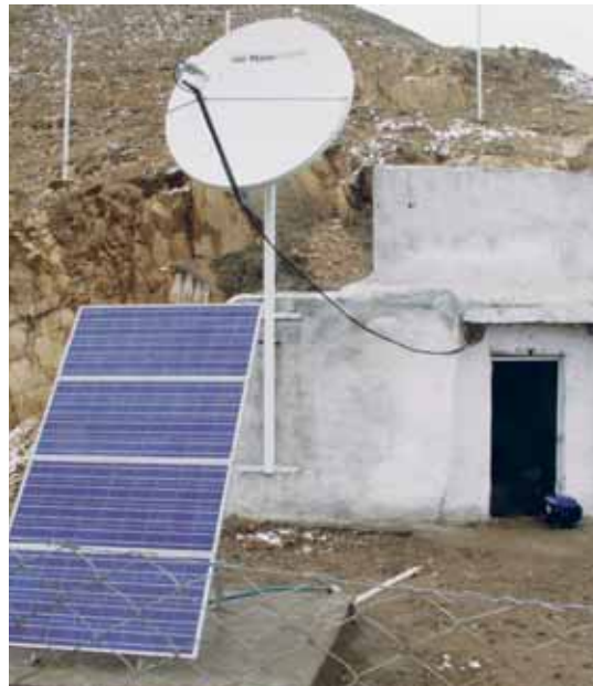
A seismic monitoring station with broadband satellite connection Location: Shartuuz, Tajikistan Photo credit: PMP International, Tajikistan
